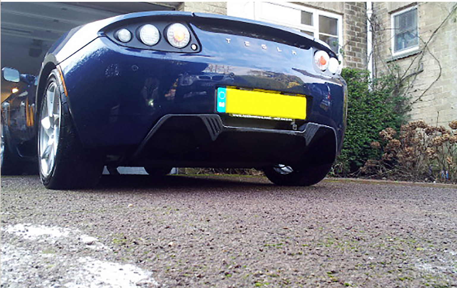
Dash CAE 3D printed a diffuser floor, seen on a Tesla underneath the license plate, on its Fortus Production System.
