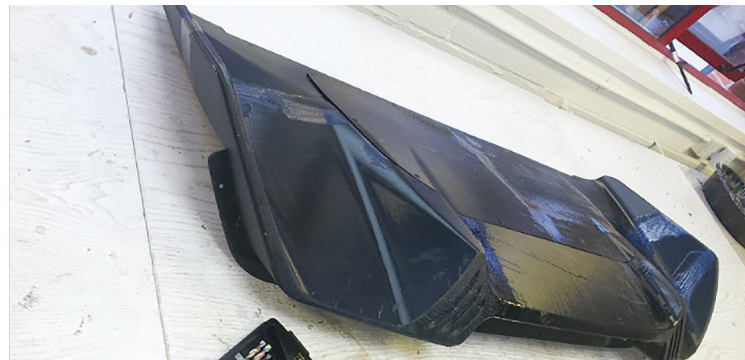
A full-size diffuser floor 3D printed in black ABSplus on the Fortus Production System
