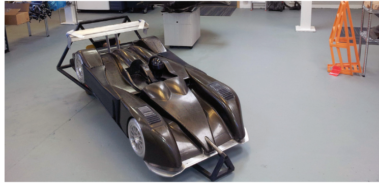
Le Mans car and Formula One chassis, 3D printed on a Fortus Production System
