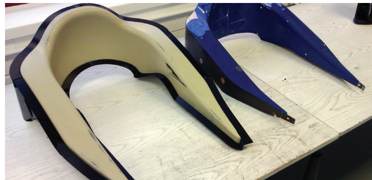
Formula One headrest, 3D printed on a Fortus Production System, to the left of the original
