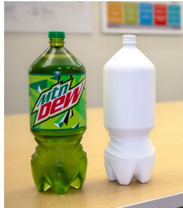
Full color 3D printed prototype next to a low-fidelity 3D printed prototype
